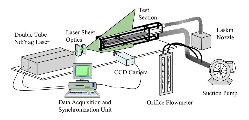
High-speed PIV system configuration with the two-pass square channel
