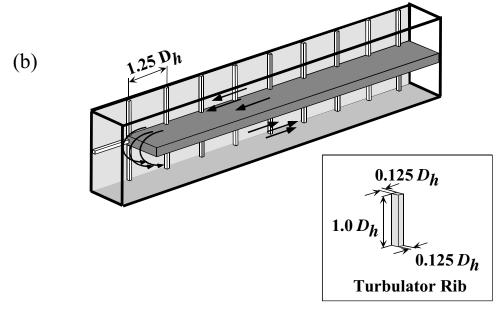
Test sections; (a) smooth wall and (b) 90° ribbed wall
